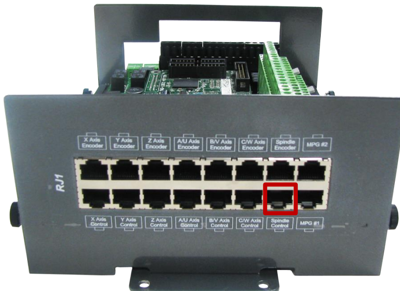
FIGURE 16 SPINDLE CONTROL RJ45 JACK
