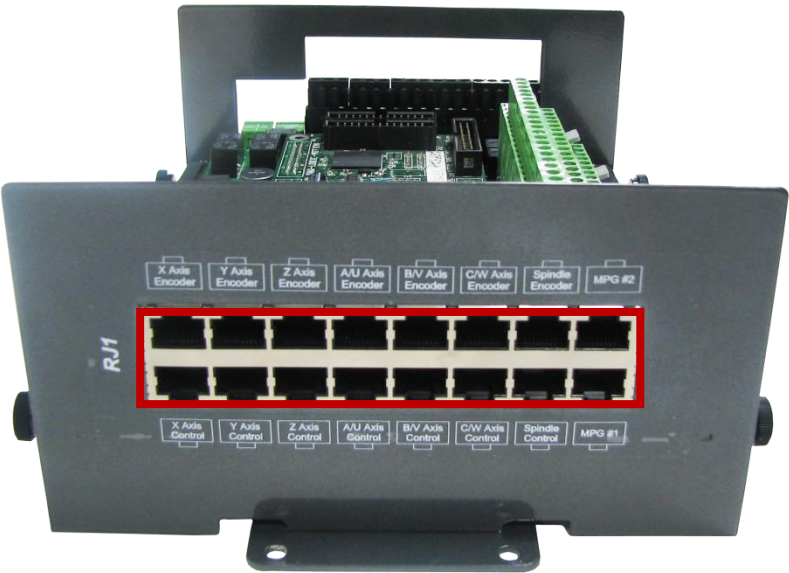
FIGURE 5 DIFFERENTIAL STEP AND DIRECTION, AND ENCODER FEEDBACK RJ45 CONNECTIONS
